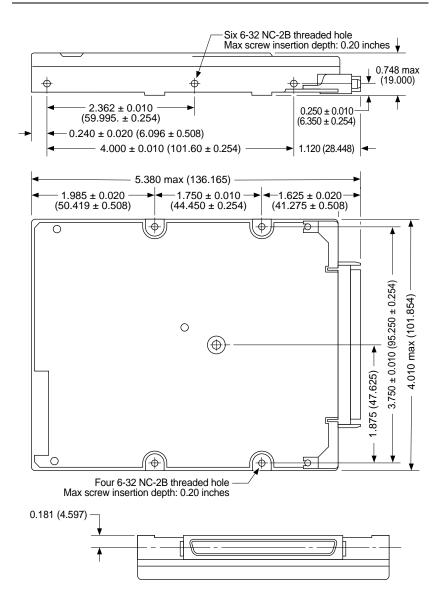
Figure 7. ST52160WC Mounting dimensions
