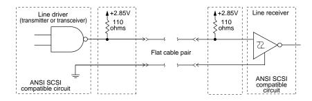
Figure 2. Single-ended transmitter and receiver
